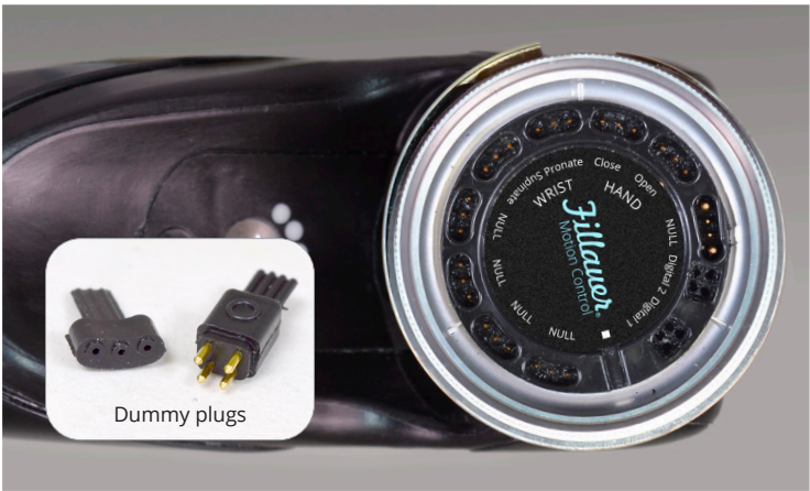
The input Manifold is marked with corresponding Degree of Freedom. Note: there is no consistency between manufacturers on polarity. Avoid grease on the label itself.
